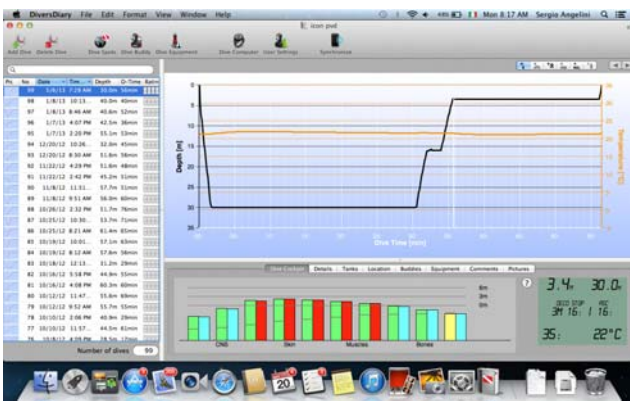
Fig. 7: Tissue tension at beginning of deco stop.
